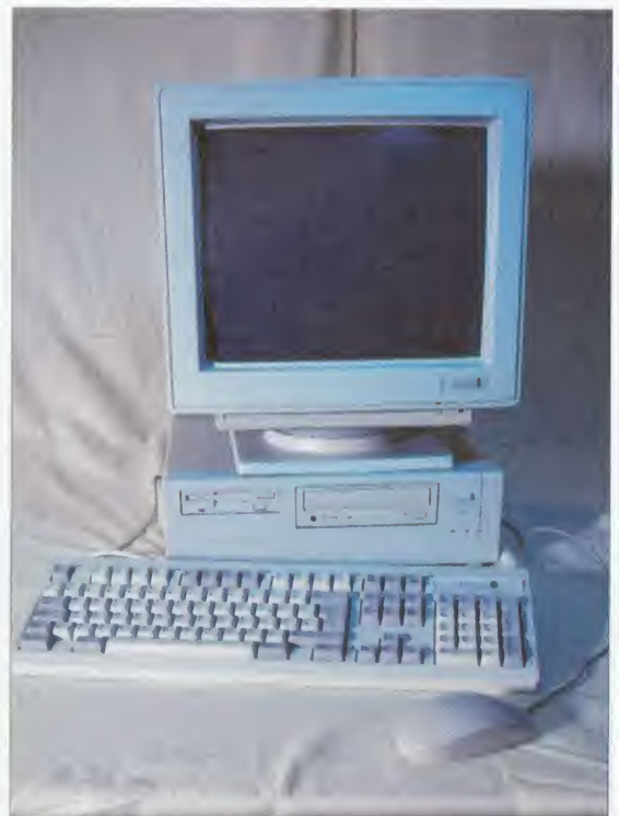
The A7000 boasts a compact and robust design. The ATAPI CD-ROM drive shown here is optional – the A7000 can take a single expansion card, but only if it has no CD-ROM drive, as they occupy the same physical space inside the machine.
